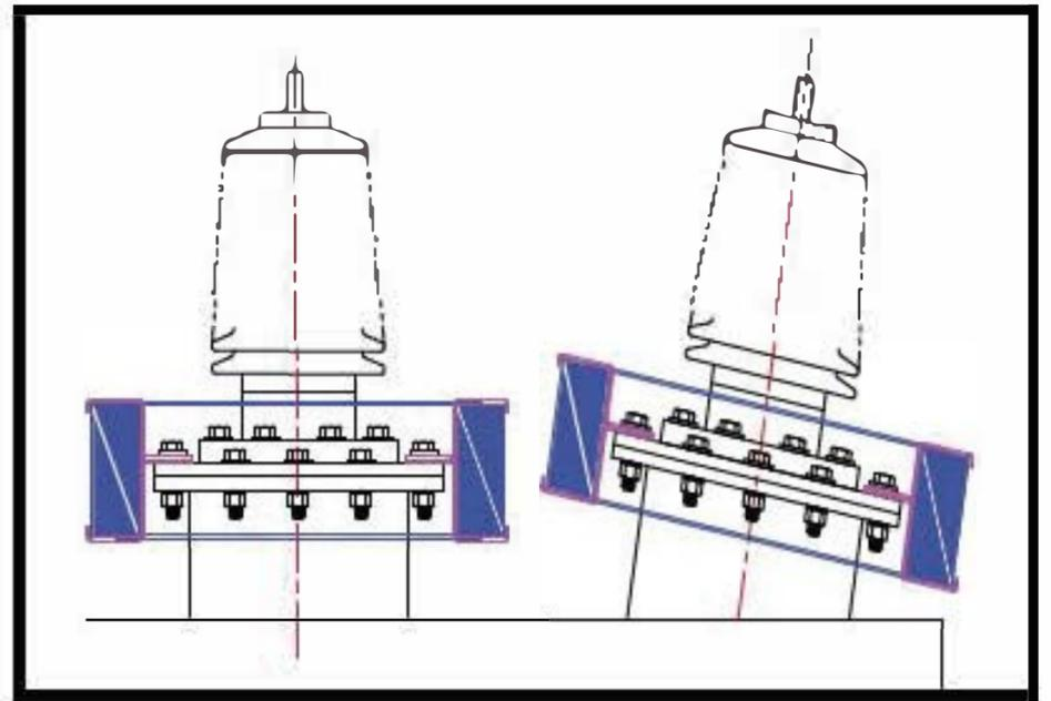
Figure 5 – Custom bracket installation mounted to and partially below the turret flange
