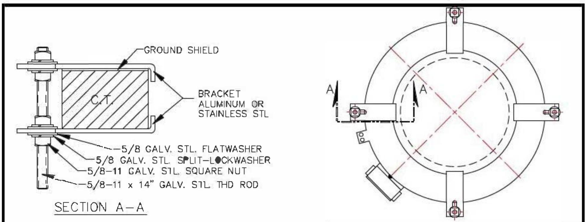
Figure 1 – Standard Mounting Brackets
