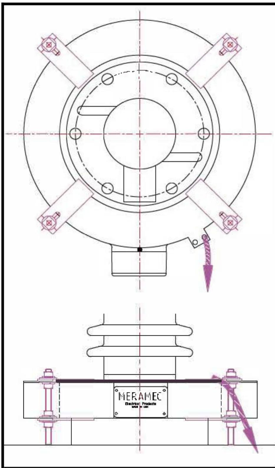
Figure 7 – Ground shield with standard brackets
