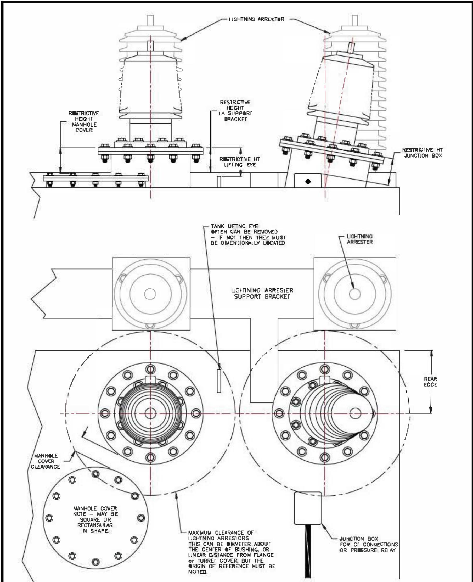
Figure 9 – Typical transformer tank top
