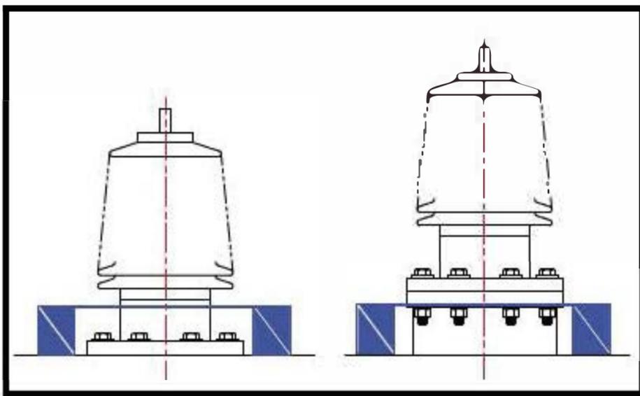
Figure 3 – Tank top mounting without brackets
