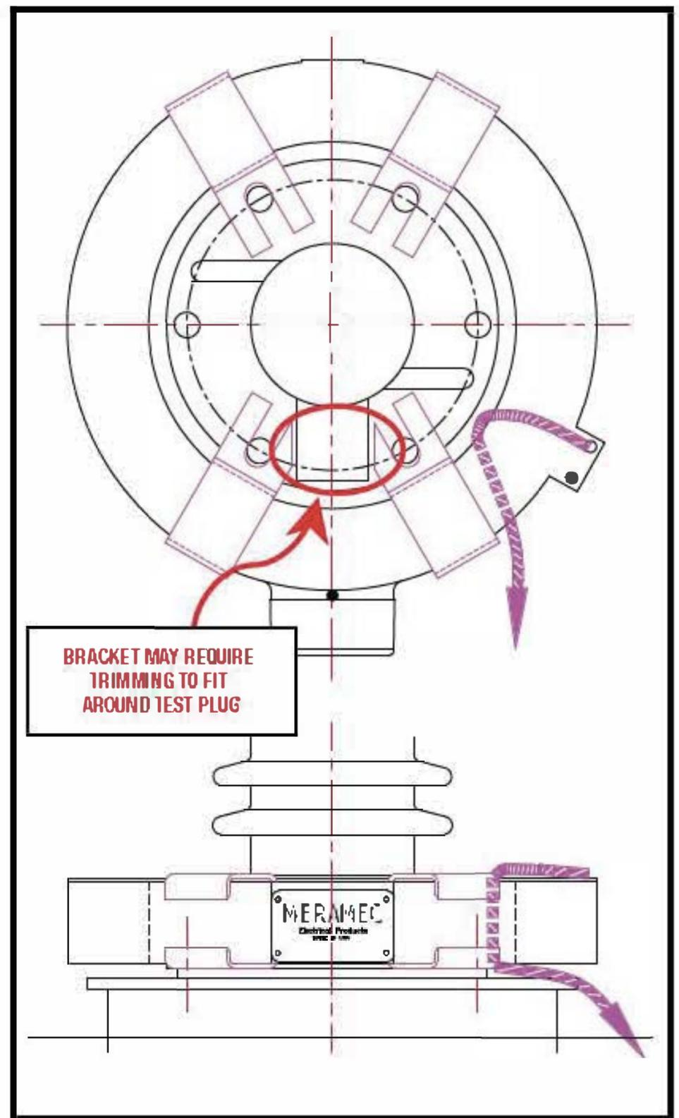
Figure 8 – Ground shield with custom brackets
