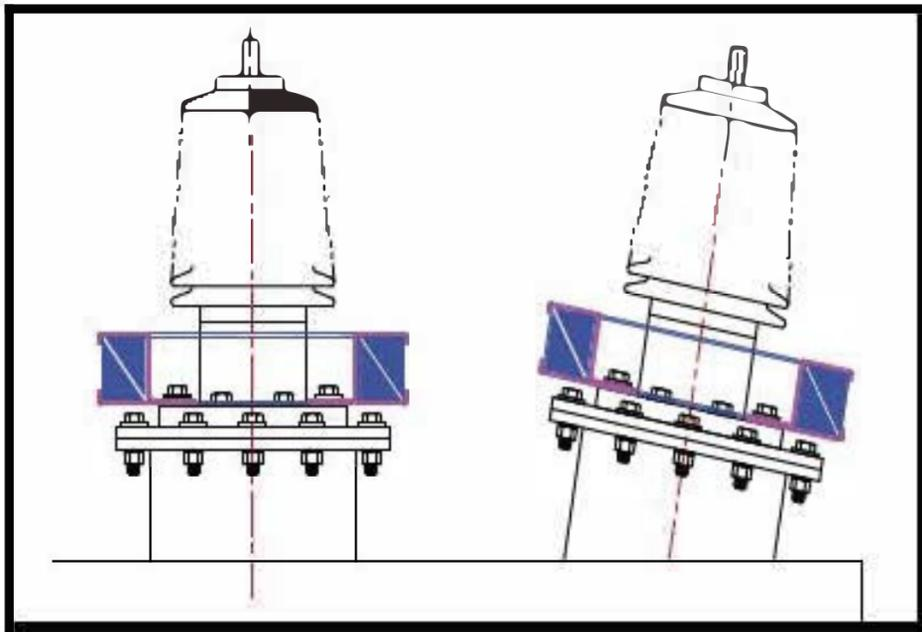
Figure 4 – Custom bracket installation mounted to and above the bushing flange
