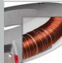
***Transformers for high current power generation applications utilize a shielded winding design*** that is an integral part of the main secondary winding. This minimizes the effects of stray magnetic flux produced from adjacent high current conductors.
